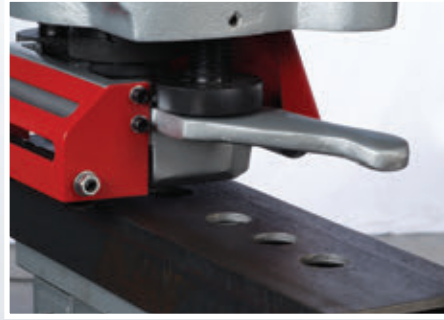
Punching channel flanges and angles
