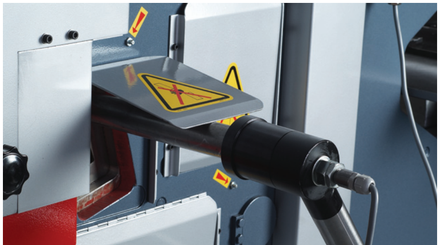
Touch and cut electrical back gauge
