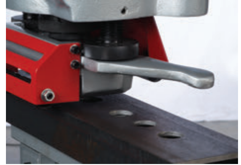
Punching Channel Flangers And Angles
